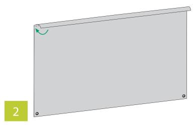
Fold graphic to create two pole pockets with a 75mm internal height.
