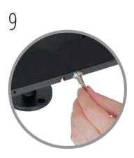
Unlock the iPad enclosure by inserting key into security lock and rotate 'QUARTER TURN ONLY' clockwise or counter-clockwise through 90 degrees which releases the locking pin. Return key back to original position to remove.
