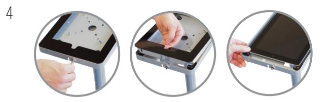
Unlock the iPad enclosure by inserting key into security lock and rotate 'QUARTER TURN ONLY' clockwise or counter-clockwise through 90 degrees which releases the locking pin. Return key back to original position to remove. Lift fascia out of enclosure, place iPad inside, gently press all four corners down into mouldings to hold.
