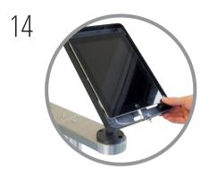
Plug charge/sync cable into one iPad and place inside enclosure, gently press all four corners of iPad down into mouldings to hold. Repeat for remaining iPad.
