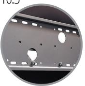
Raise screen mount so bottom holes are above the lower horizontal rail in aperture. Re-insert 2 screws through lower/inner mount holes (4 openings from either end of the screen mount) and clearance holes in 2 off 260mm connector bars adjacent to mount.
