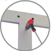
Connect second horizontal 1500mm rail assembly (H), using the expanding clamps, to top of assembled verticals (V, V1 and V) ensuring that the graphic fixing strip is at the bottom. Tighten grub screws on vertical rails to secure. This completes the bottom section of the framework.
