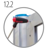
Affix the top section framework into the same channel as the bottom section ensuring graphic fixing strips are all on the same side of the system. Leave a gap of 60mm in between bottom and top framework assemblies and tighten all grub screws in horizontals (H and H1) to secure to post.
