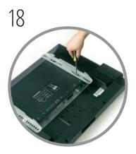
With the elongated holes on the mounting arms lowermost, align arms centrally with 4 off fixing points on rear of screen equidistant from the top. Insert 4 off screws with suitable washers and tighten.
