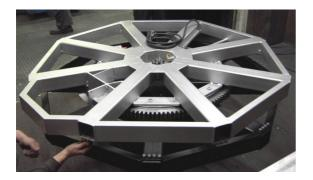
Maximum centric load: 3,000 kg / 6,600 lbs Turn plate: Ø 1250 mm Height of turntable 230mm
