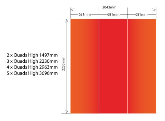
An Easy Tower Circle is covered with three graphic (or fabric) panels using 680mm hookstrips to attach panels to frames.
