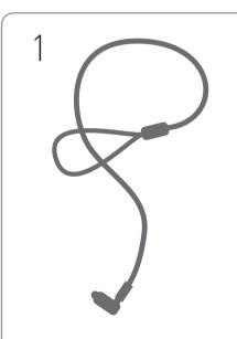
Lasso the security cord to a stationary anchor point, by passing the lock body through the looped end of the security cable.
