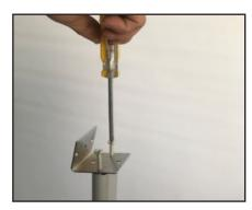
Using the two long screws through steel holding to pole groove and take screwdrivers to fit them in tight.
