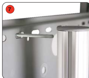
7 Attach LCD mount to 50mm round posts with M6 x 70mm screws, flat washers, spring washers, and thumb wheels.
