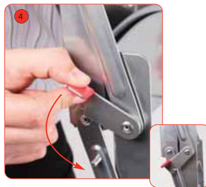
Once unit is fully extended, push the locking arm forwards and secure into place by slotting the hook over the locator pip.
