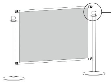
Cross bar end fits into hole in post collar. Cross bar end locks into position by pushing flexible tab past collar.
