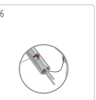
Loosen and slide connector bars halfway out of 1m post. Tighten grub screws of connector bars positioned in post channel to secure
