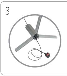
Feed figure-8 head of power lead through bottom of post and profiles assembly, leaving approximately 1m of cable at bottom.
