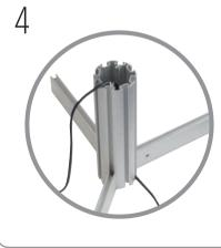
Stand post and profiles assembly upright ensuring lead is kept clear of foot screws.
