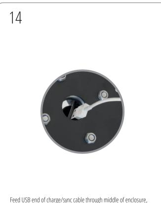
Feed USB end of charge/sync cable through middle of enclosure, below pin, so it protrudes from bottom of support column.
