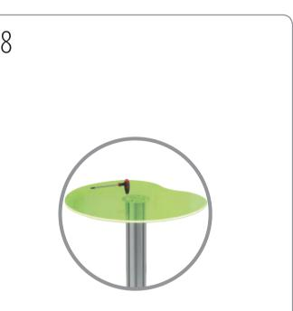
With countersunk holes in the Podium tops uppermost, align with holes of circular plates and fixings in the top of remaining small, medium and large posts. Fully insert 4 screws in each to secure.
