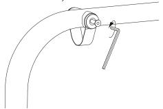
Locate panel onto the panel hanging clips. Reassemble the panel hanging clips using the screws and fixings.
