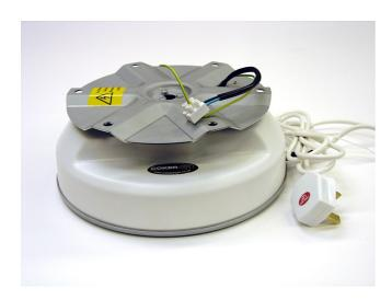
The turntable TTC 250 for 25 kg (55 lbs) centric load has a turn plate with large diameter, fixed hollow shaft in the centre and collecting ring option. It provides a wide range of applications. It is appropriate for fix installed lighting on a tube in different lengths. Power supply, lamp holders or devices for fluorescent lamps can be provided standard (i.e. for light cubes).
